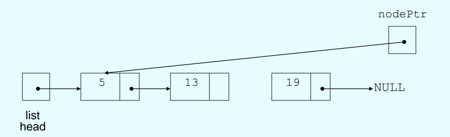
nodePtr points to the node containing 5, then the node containing 13, then the node containing 19, then points to NULL, and the list traversal stops
