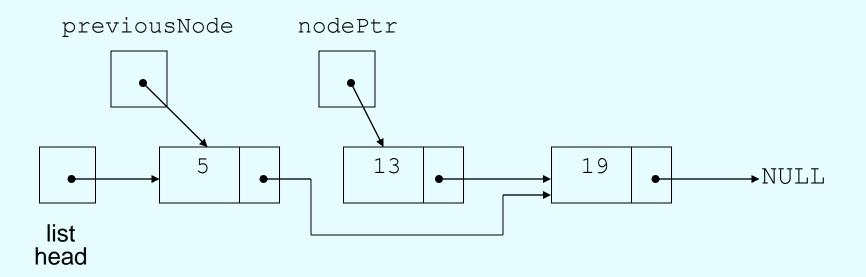
Adjusting pointer around the node to be deleted
