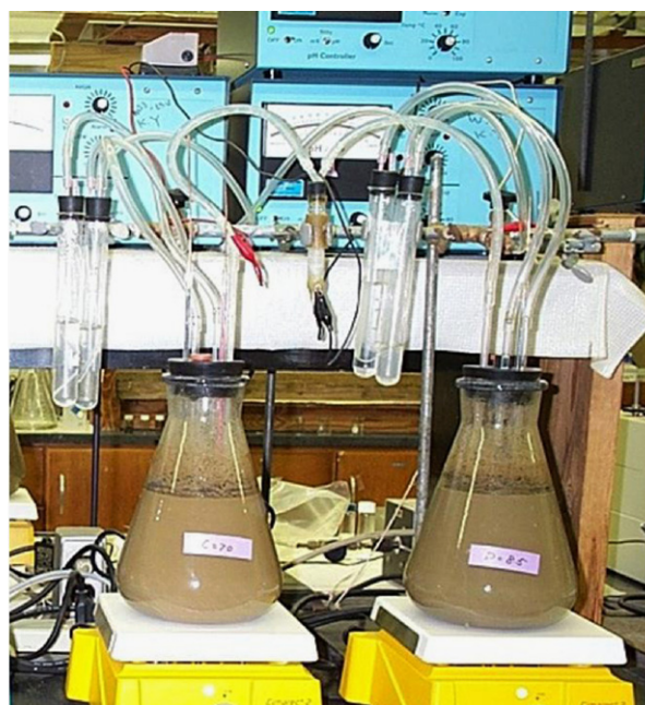
Fig. 1. Basic components of a soil microcosm, a schematic (left) and a photo (right).
